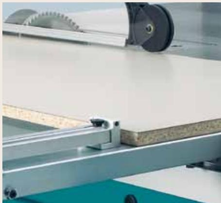
T7068 Second support with T7055 parallel cutting stop
