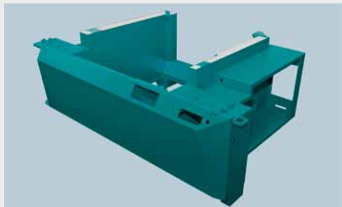
[1] T70 steel/concrete composite machine frame
