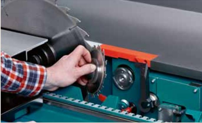
T7023 Electrically adjustable 3-axis scoring saw unit
